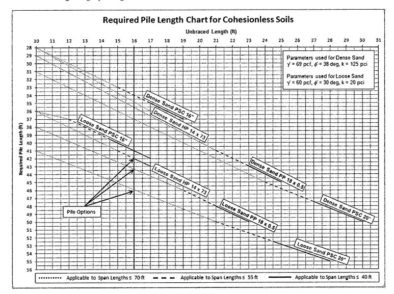
Based on the given information and the *Required Pile Length Charts*, there are three piles that may be used. These three options are listed below and also shown on the chart above. The 16" Prestressed Concrete Pile is not an option because in loose sand with an unbraced length of 16 ft, it can only be used for average span lengths less than or equal to 40 ft.
